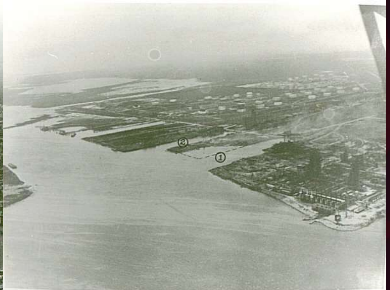
FIG. 6. General view of damaged area looking to the southwest. Note smoke from burning flume in ruins of Warehouses "O" and "A" in center portion. Locations of S. S. GRANDCAMP and S. S. HIGH FLYER at 1 and 2 respectively. This picture was made 3 days following original explosion.
